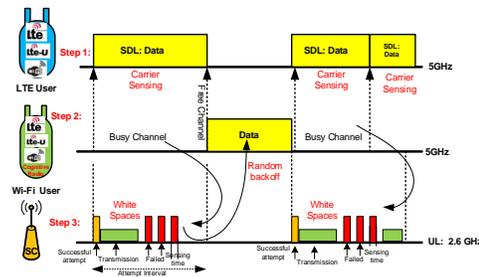
Fig. 2. Channel access mechanism of WiFi-Lic
